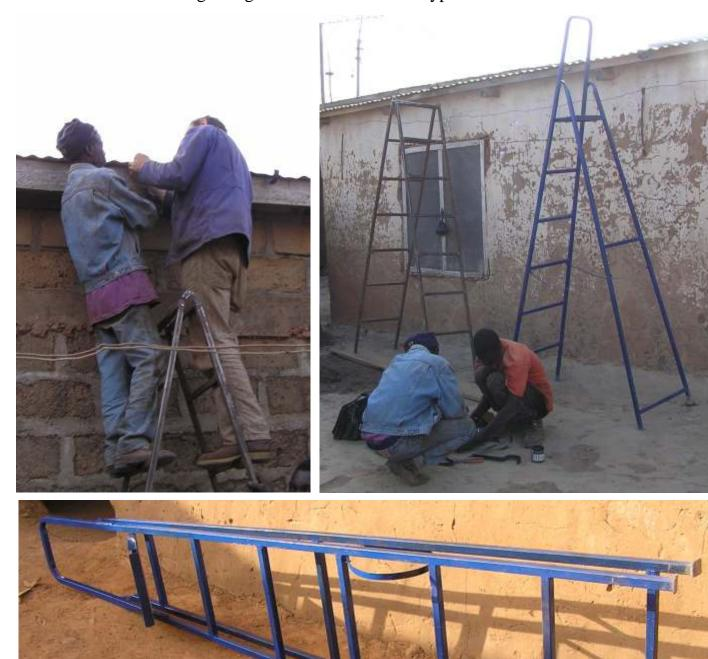
Materials: Pipes 25x25x1.5 Platform: sheet 2 mm Straps 20x1 mm Hinches: flat bar 20x4
